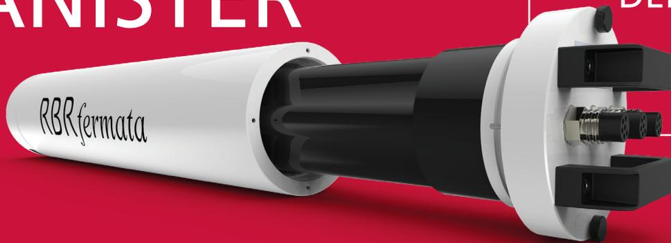
The RBR*fermata* battery canister is available in three pressure ratings (750m, 4000m, and 10,000m), and is capable of extending deployments for all RBR instruments and any other devices requiring a nominal 12V supply. Three MCBH connectors are mounted on the top end-cap, and the battery pack design accommodates 56 D-cells, soldered with reverse- and short-circuit protection, in a single wrapped pack.
