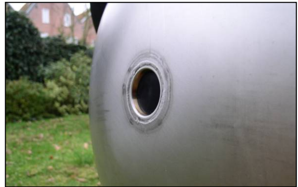
Recessed transducer in the hull.
